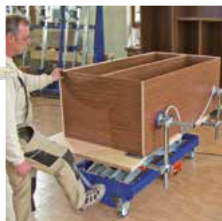
The hole plate can be used for pressing and assembly
