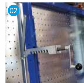
Hold-down clamp quick adjustment (also applies to RPG-NH) 01 02
