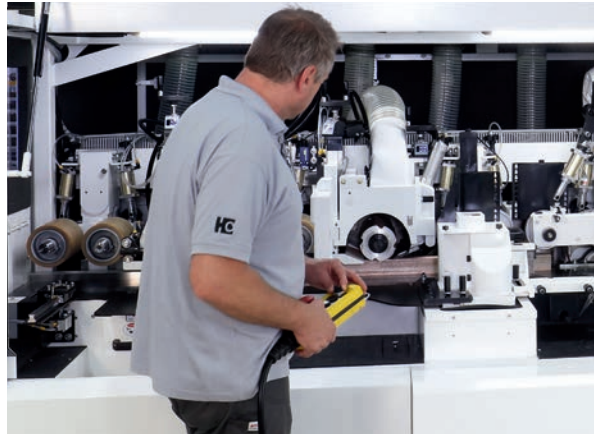
Ergonomic remote control for quick and automatic adjustment of selected spindles
