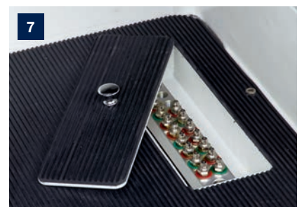
Accessible central lubrication at machine front
