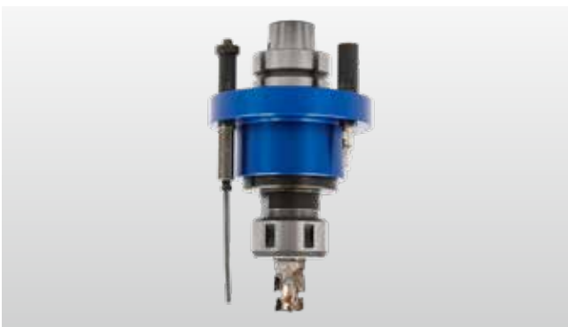
Trimming tool holder with jet for compressed air and fluids: For trimming operations combined with compressed air feed, for example for tool cooling when processing plastics or to improve chip disposal when trimming deep grooves.
