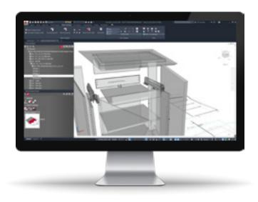
Design assistants and optimum operating sequences ensure simple and rapid design. Thanks to the parametric design approach, details, entire assemblies or room plans can be changed and recalculated at any time.
